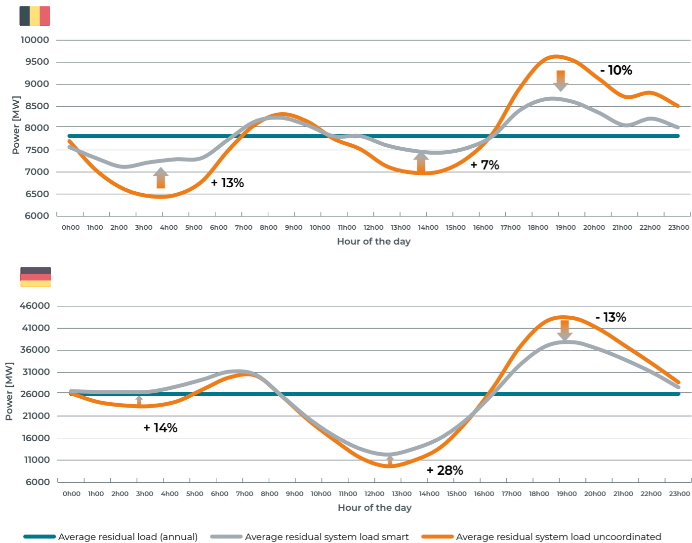
Figure 8 : The impact of electric vehicles on residual load for both Belgium and Germany in 2030
