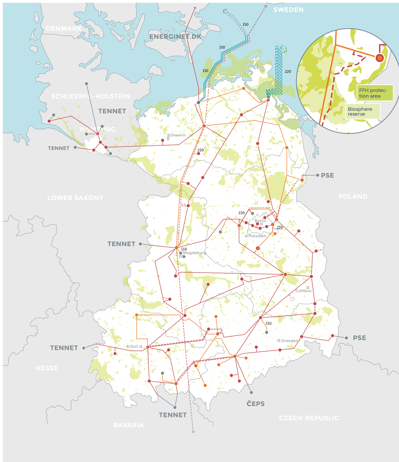
There are many different protection zones in the 50Hertz grid area, which are recorded in a cadastre. The FFH protection zones, national parks and biosphere reserves are displayed in the picture. Among other things, the grid area contains many bird sanctuaries, which 50Hertz makes sure to protect when building new lines.
