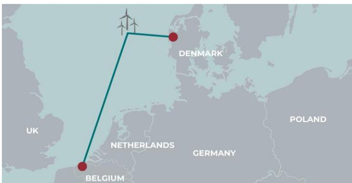
When the interconnector between Belgium and Denmark is completed, the cable will run through the territorial waters of four countries: Belgium, the Netherlands, Germany and Denmark. Stretching over 600 km, it could be the longest subsea direct-current (HVDC) cable in the world.
